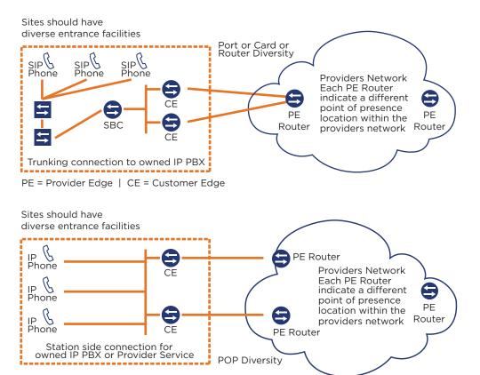
Figure 5 below represents another redundant design to avoid call failures. Although the diagram shows trunk side connectivity for a company-deployed IP-PBX, the remote site shows how the design would work for one provided by a third-party as well. This is an ideal design scenario, but acceptable availability levels can still be achieved if the level of redundancy in this design is not available at all sites.
